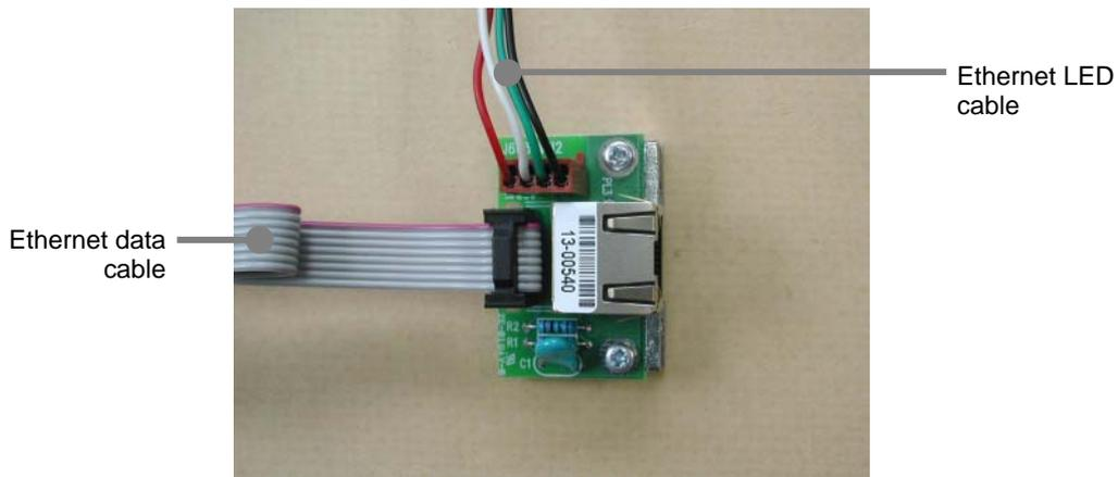
For all connections, the red wire on the cable is pin 1. Pin 1 on each connector is marked on the board.
